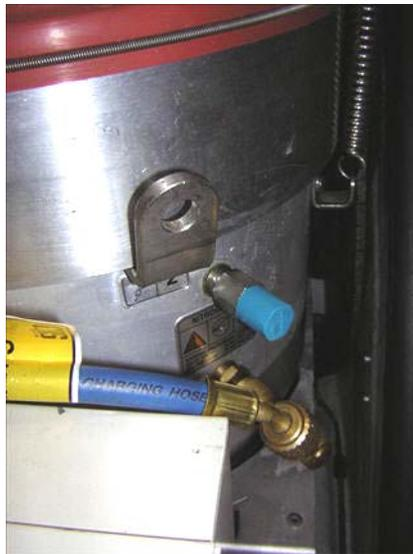
5. Open the secondary valve and check the pressure on the gauge.
