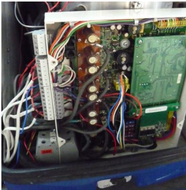
2. Remove all wires from the terminal block at the left side of the electronics. Careful with the voltage sensor wire (nr. 9) which is still connected to the battery bank.
